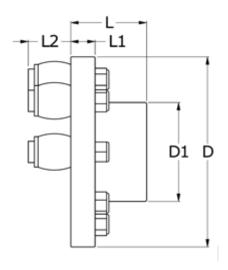
D = 105 D1 = 59 L = 45 L1 = 12 L2 = 30 Max bore = 38 Torque (N m) = 200
